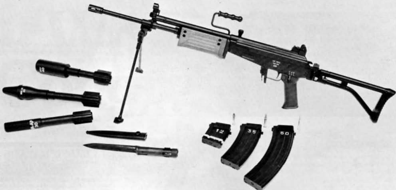
Above: The Galil is shown here with all of its basic combat accessories: three different grenades, bayonet and scabbard, magazines of three different capacities and carrying handle. With bipod extended, it assumes capabilities of a squad automatic weapon or LMG.
