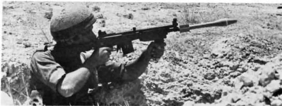
The Galil handles a wide variety of grenades. A special magazine is required for grenade launching cartridges.
