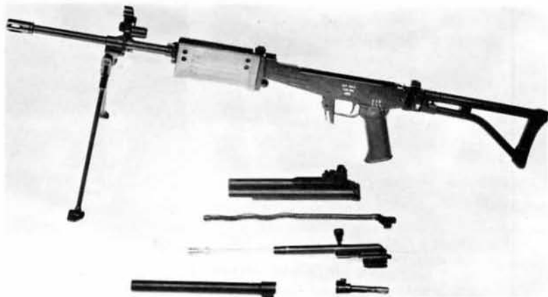
Here the Galil is shown field-stripped for cleaning and maintenance. In this photo, anyone who is remotely familiar with the AK47 will immediately notice that the parts, for all practical purposes, are identical.
