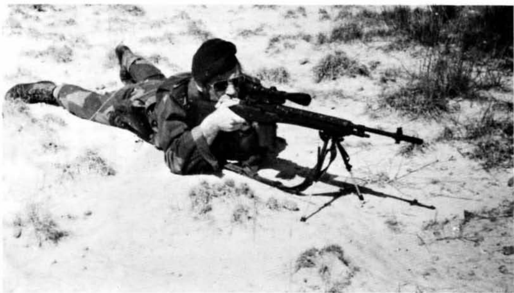
A Harris ultra-light, spring-activated Model 1A bipod is attached to this M1A/ART combination. The bipod can be ordered from Harris Engineering, Inc., P.O. Box 305, Fraser, MI 48026
