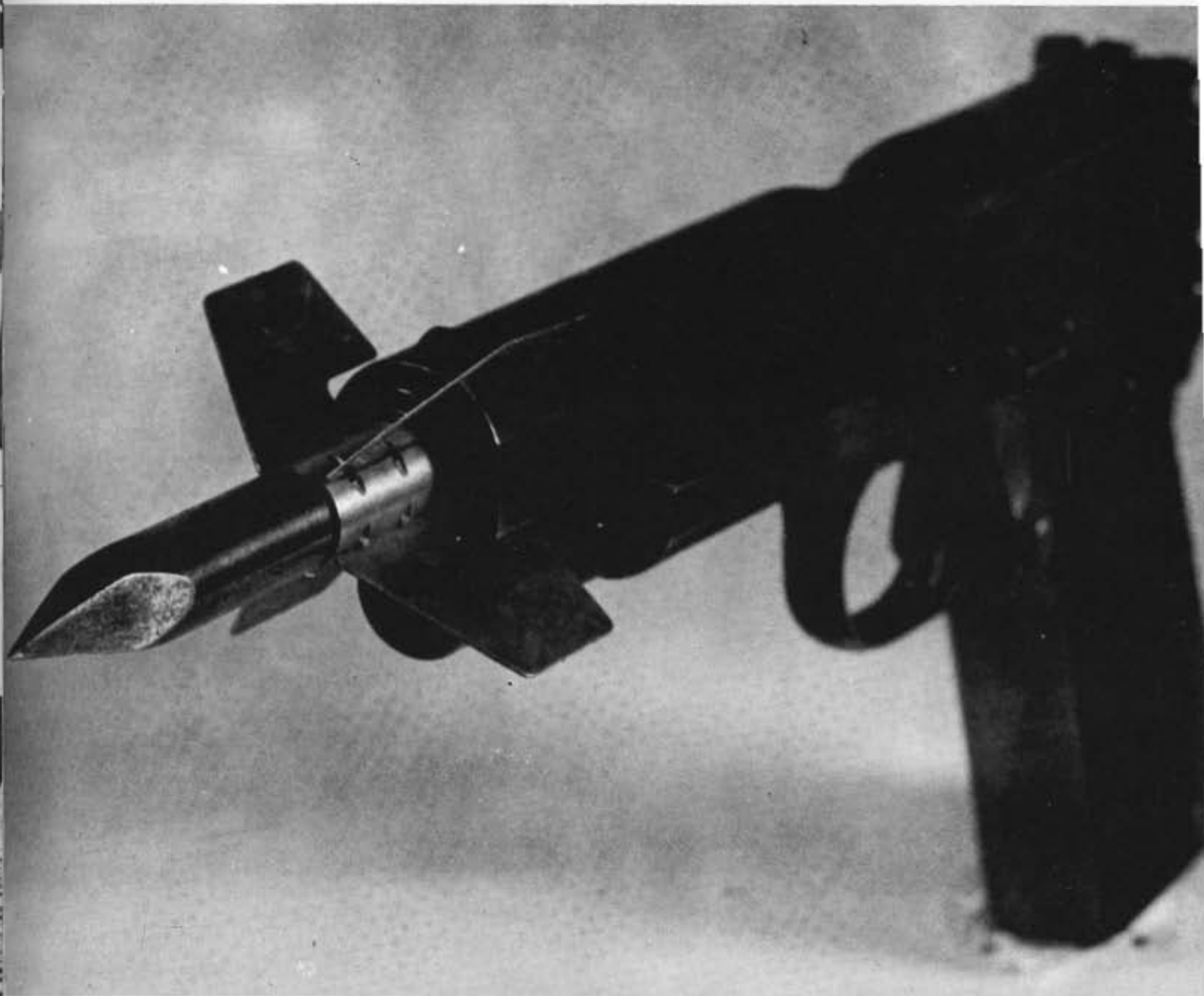
A M1911A1 .45 cal. automatic was modified to accept a spigot, over which fit a dart-like projectile. Propellant was contained in the projectile's shaft.
