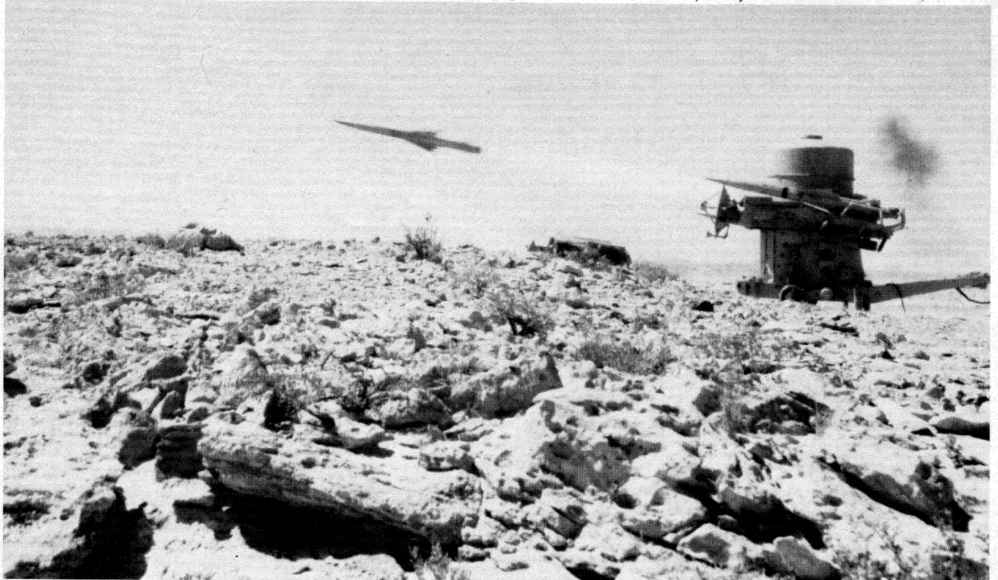
A Rapier of the Omani Defence Force. The Rapier system has been in service in Oman since 1976 using the optical system for airfield defence. An order has now been placed for the blindfire Radar which will provide round the clock capability in all weather.
