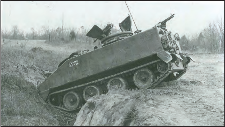
Figure 50. An M114 vehicle in Vietnam showing its difficulty with cross-country mobility.
